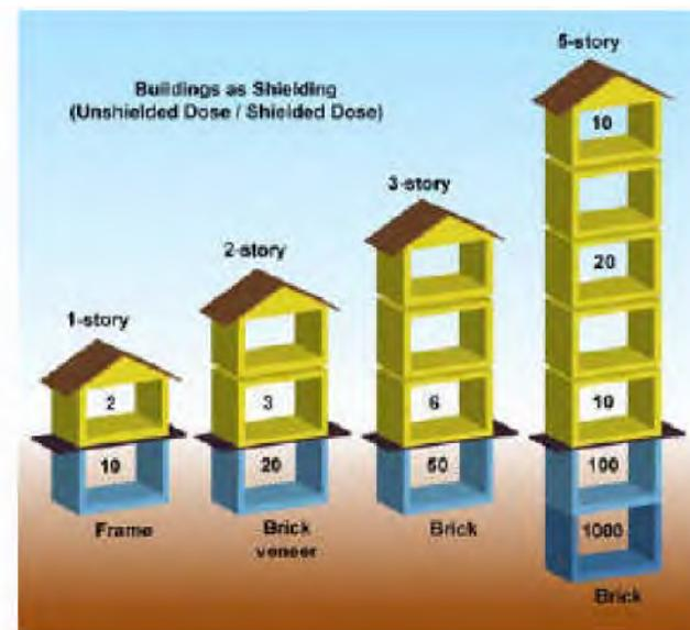
Slide 8b Building as shielding: numbers represent a dose reduction factor. A dose reduction factor of 200 indicates that a person in that area would receive 1/200<sup>th</sup> of the dose of a person out in the open.
