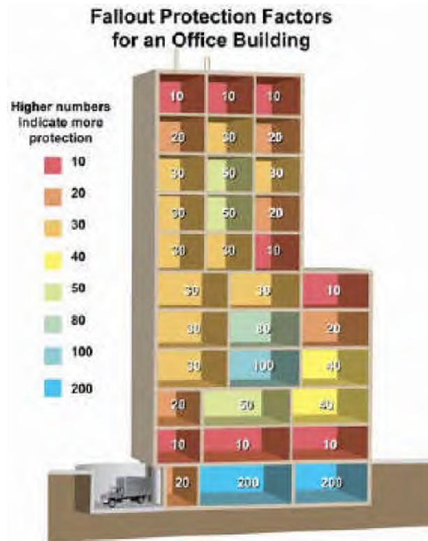
Slide 8a Building as shielding: numbers represent a dose reduction factor. A dose reduction factor of 10 indicates that a person in that area would receive 1/10<sup>th</sup> of the dose of a person in the open.
